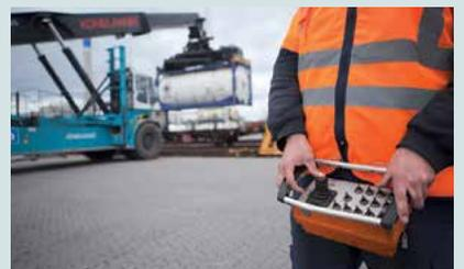
Remote control unit for rail and barge handling
