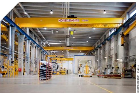
technology. For the heaviest lifts, the plant was provided with a high-capacity SM crane with a lifting capacity of 130 tons. It had the Extended Speed Range (ESR) feature to speed up the lift when the hook is empty or with a small load.
