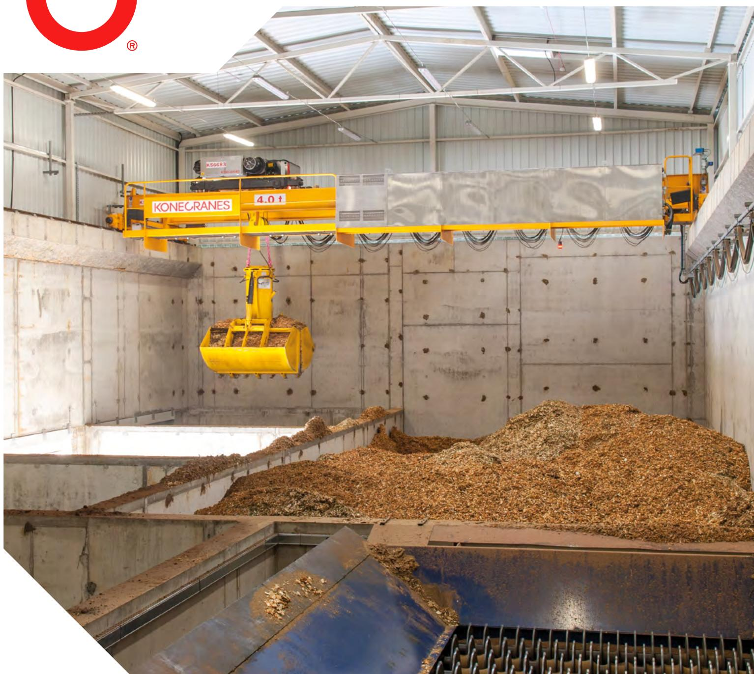
New Heat, a recognized EPC provider of boiler houses and combined heat and power (CHP) plants, constructed, for Lorizon Energy, a new biomass power plant located in Kaunas, Lithuania. The plant is equipped with a 10 MW boiler house, where heat is produced. The plant is capable of using three different types of biomass – straw pellets, wood chips, and peat. Each fuel type can be used separately or mixed together for maximizing efficiency.
