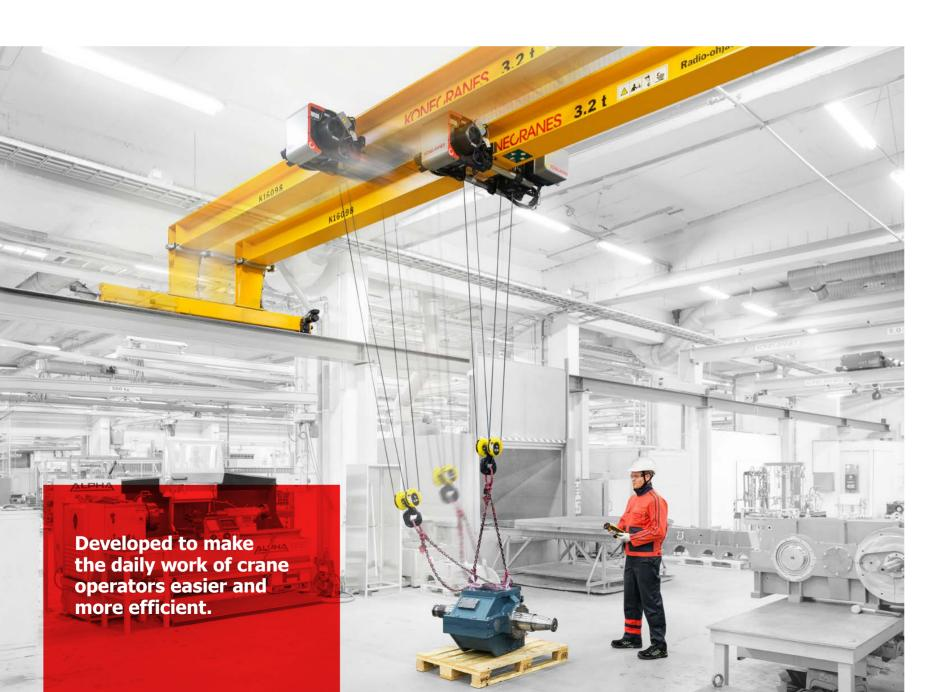
**ASSISTED LOAD TURNING** helps turn the load by keeping the ropes straight and eliminating side pull. This function makes one of the most challenging crane operations easier and less risky. It speeds up duty cycles, extends crane lifetime and simplifies crane operation.
