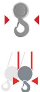
**SWAY CONTROL** limits load swing by controlling the bridge and trolley acceleration and deceleration. Sway Control allows faster load handling and more precise positioning. This feature also reduces the risk of damage to the load, crane and surrounding area.
