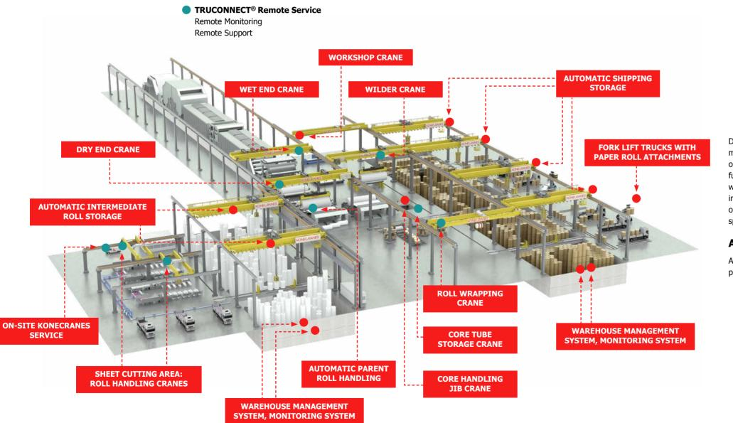
Drawing on our long experience with paper manufacturing, we have specially designed our ASRS for paper storage facilities. It uses fully-automated cranes to help speed up work cycles, reduce roll damage and track inventory. Without the need for forklifts or open aisles, you can optimize your storage space and minimize your labor costs.
