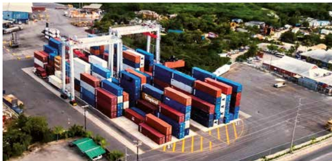
The Port Authority of the Cayman Islands (PACI) operates Konecranes BOXHUNTER RTGs at this inland storage facility on Grand Cayman. The cranes were delivered in 33 containers and swiftly commissioned. They're equipped with Smart Features that speed up the positioning of containers and increase their landing accuracy for fast cycle times.
