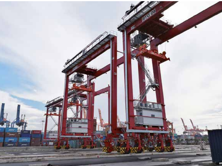
Konecranes Noell RTGs at Dinh Vu Port, Haiphong, Vietnam. They are 8-wheel RTGs lifting 1-over-5 containers high, and fully electric powered by cable reels.
