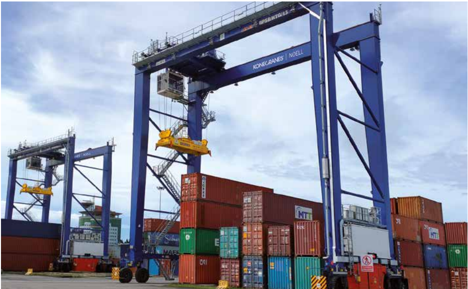
Konecranes Noell RTGs at Bintulu Port, Malaysia. They are 8-wheel RTGs fitted with the Konecranes Core of Lifting for hoisting, trolley and gantry movement. Bintulu Port is East Malaysia's largest container port and the nation's only liquefied natural gas (LNG) export gateway. It's one of the largest LNG export terminals in the world.
