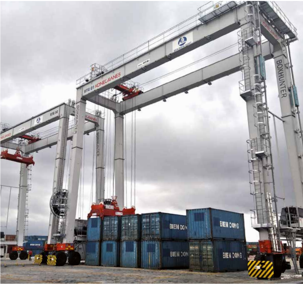
BOXHUNTER has a system of counterweights that reduces energy costs because it eliminates the weight of the spreader – amounting to a 25% lighter load with every lift.
