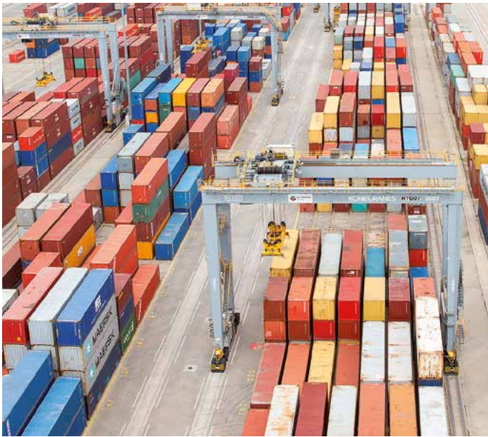
Konecranes RTG at DP World Yarimca in Turkey, in fully electric operation powered by a cable reel system.
