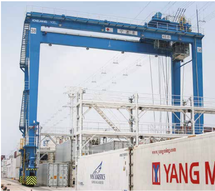
A Konecranes Noell RTG in action with an additional power option: overhead electrical trolley power.
