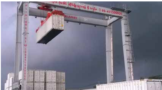
CGM Logistics in Myanmar operates BOXHUNTER at a special inland logistics facility. BOXHUNTER is part of a new business concept, where customers rent storage space in portions of containers that are stored in an outdoor yard. The operator's ability to jump in and out of the machine at ground level is central to the concept.
