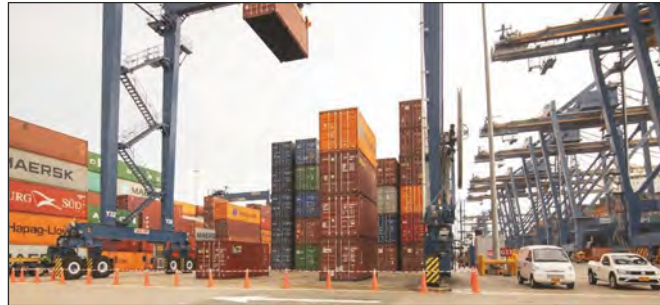
The test site for the first two automated RTGs at the Contecar facility
