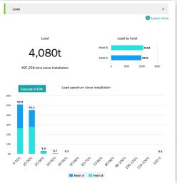
This section shows the production volume of the crane or individual hoist.
