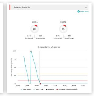
Portion shows the calculated remaining service lifetime of hoist contactors – up/down direction, fast speed and brake contactors. When the value approaches zero, contactors should be changed. The service lifetime is directly influenced by the usage rate of the hoist and, most significantly, by the use of jogging/inching.
