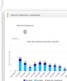
The chart shows the ratio of low and high-speed operation of a 2-speed motor and the number of over temperature episodes in the same period.
