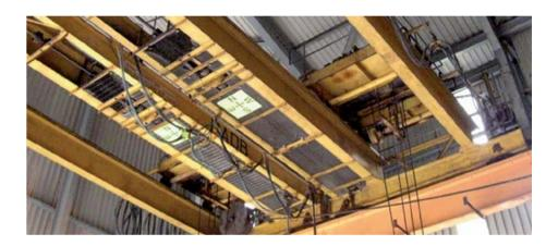
Modernization of its 20-ton pneumatic maintenance cranes has improved safety and reliability and extended crane life. Inspection and maintenance contracts make long-term use of Konecranes expertise and global service.
