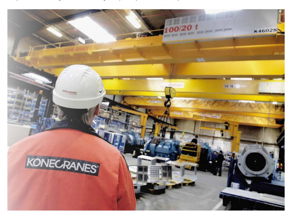
sway control limits load swing by controlling the bridge and trolley acceleration and deceleration. Sway Control allows faster load handling and more precise positioning. This feature also reduces the risk of damage to the load, crane, and surrounding area. ACTIVE SWAY CONTROL is also designed to dampen existing load sway.
