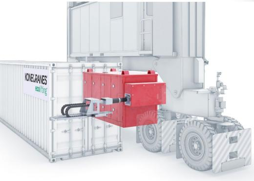
Docking at the charging station is a simple matter of gantrying the B-RTG to the station, where the charging connection is made. This can be done in automated mode, in ARTG operation, or in manual operation. Regular containers can be stacked on top of the charging station, which is just another container as far as stack operations are concerned. Charging can also be done via manual connection to the port mains. This is an easy-entry solution for e.g. intermodal terminals.
