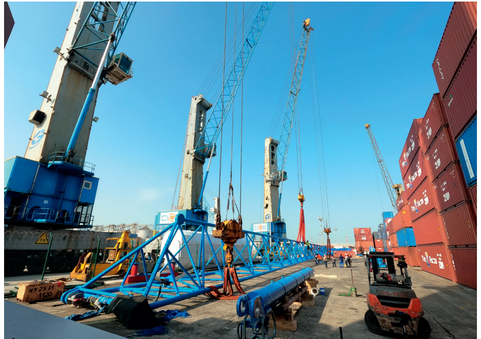
The existing fleet of Konecranes Gottwald Mobile Harbor Cranes helped to assemble the new Generation 6 crane
