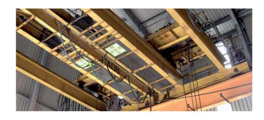
The modernization of its 20-ton pneumatic maintenance cranes has improved safety and reliability and extended crane life. Inspection and maintenance contracts make long-term use of Konecranes expertise and global service.
