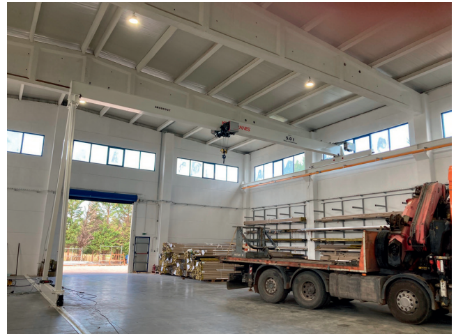
Semiportal 5 ton Single girder Crane with 14m span
