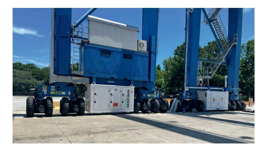
At the Wando Welch Terminal in Charleston, South Carolina Ports (SC Ports) has had 12 of their Konecranes RTGs upgraded with an EPA-approved Konecranes hybrid retrofit. These cranes now have reduced fuel consumption and lower carbon emissions with easier maintenance while retaining the same level of operational performance.
