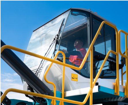
A panorama roof window and large, lowered windows with no corner posts lead to superior visibility.
