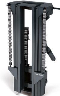
Triplex, 3-stage with freelif
