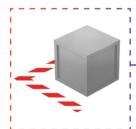
**WORKING LIMITS** creates temporary "virtual walls" which limit where the crane can move. It is a flexible safety tool in which settings can be easily changed for different tasks, shielding areas where people or equipment are located.
