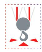
**HOOK CENTERING** eliminates side pull during lifting by positioning the bridge and trolley directly over the load. This reduces wear and tear on components, faster duty cycle times and easier operation.
