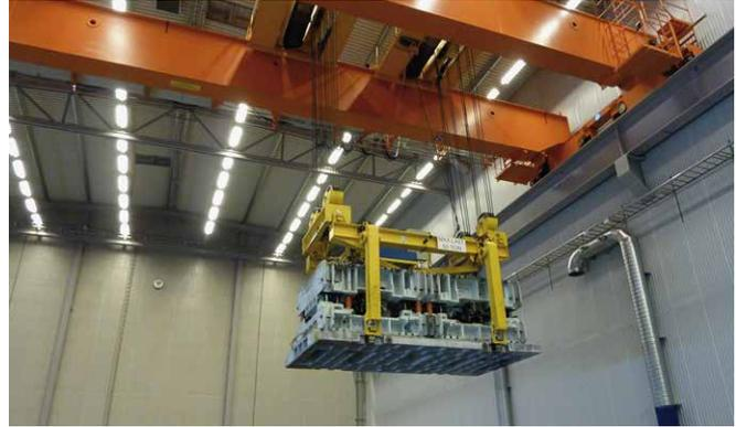
Cranes can also be equipped with a Die Gripper (or Die Lifter). The operator can control the width and length of gripper by a radio controller. Gripper legs are controlled by inverter. The needed positioning accuracy of a Die Gripper Crane is usually about +/- 20 mm realized with the following measures:
