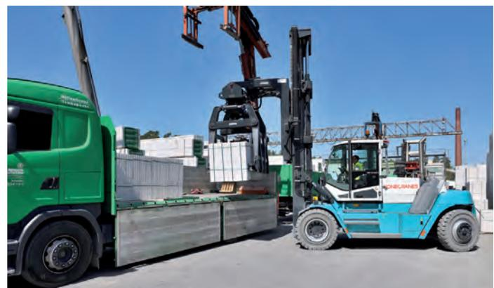
Konecranes Liftrucks has designed two heavy-duty lift trucks with stone stack gripper for Heidelberg Kalksandstein GmbH in Durmersheim, close to Karlsruhe in Germany.
