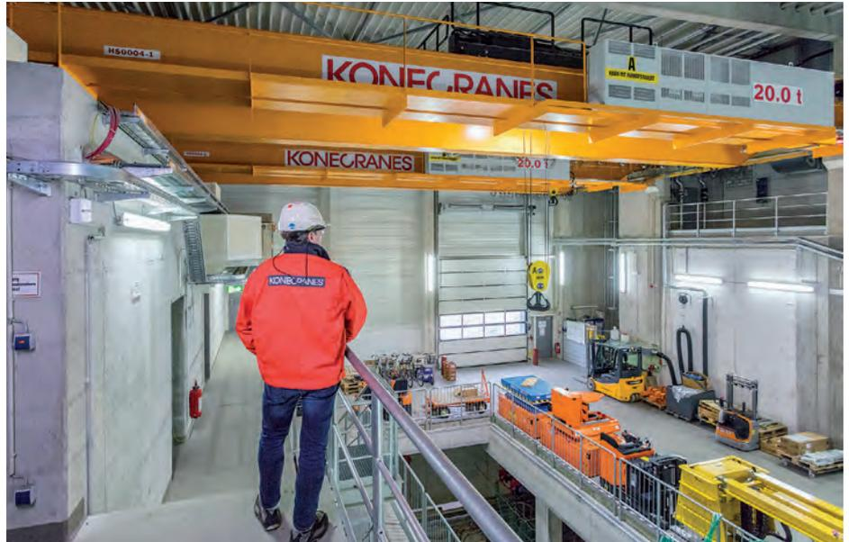
components and large concrete slabs. The two CXT double-girder overhead cranes at the tunnel entrance also save space thanks to their rotated cable drums and can work synchronously in tandem mode.
