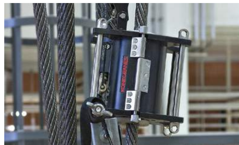
RopeQ detects internal broken wires that are not visible to the eye and would be missed by traditional inspection methods.
