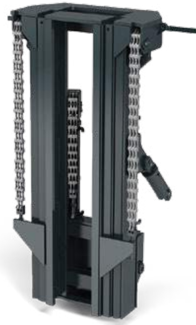
Triplex, 3-stage with freelif
