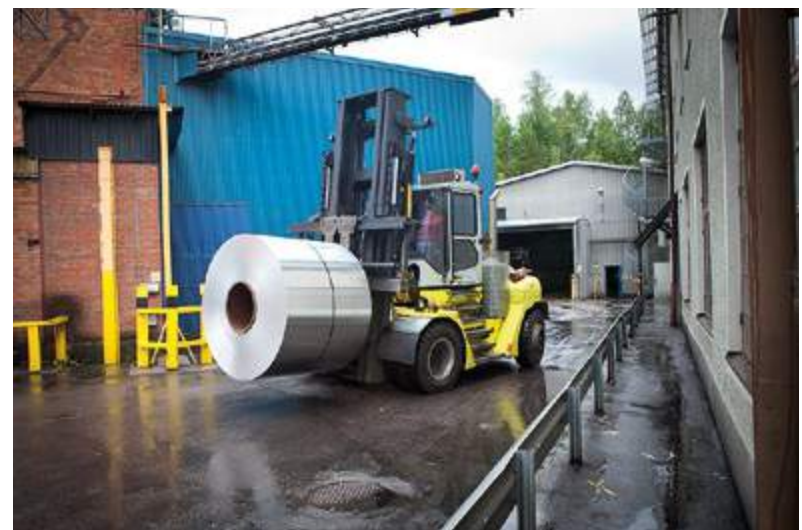
Sapa Heat Transfer AB in Finspång, Sweden, operates a fleet of 10-ton Konecranes fork lift trucks in their warehouse and shipping operations. The trucks were designed specially to Sapa requirements.
