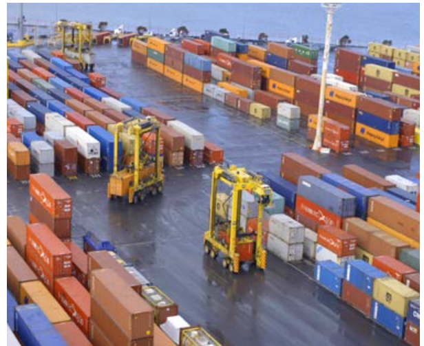
Manual 1-over-2 Konecranes Noell Straddle Carriers working in the Port of Auckland. Automated straddle carriers (A-STRADs) from Konecranes will stack containers 1-over-3 here in the future.
