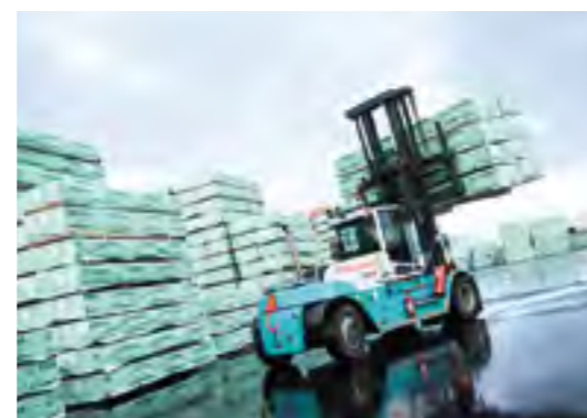
FORK LIFT TRUCK WORKING IN A SAWMILL , lifting 2 to 4 wood packages at a time, 8–16 tons. Different attachment combinations available including special fork leveling carriages.
