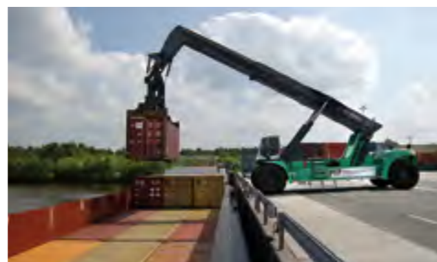
THE BIGGEST REACH STACKERS IN THE WORLD for barge loading of containers and other cargo, with an outreach 3 containers wide. This truck can do yard stacking and load railcars and river barges – 3 functions in 1 truck. Very high lifting capacities.
