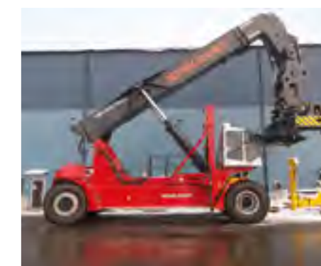
SMV 4542 TBX4 BH REACH STACKER , Terminal de Seine, France. Container barge handling. Equipped with a vertically movable cabin and ELME 817 spreader with overheight folding legs.
