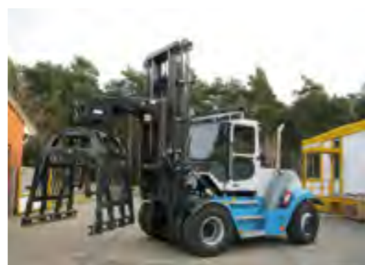
CONCRETE PRODUCTION of various kinds. Loading trucks, extra-wide carriage (7 m) with 4 forks and side-mounted cabin for extra visibility, SMV 37-1200 C and 50-1200 C.
