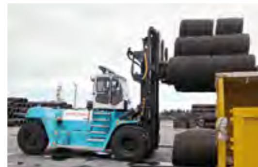
FORK LIFT TRUCK WITH TRIPLE COIL RAM mounted on a fork shaft for handling steel wire. The quick-change fork shaft makes it possible to swap between various forks, coil rams and other attachments very quickly. Capacities from 10 to 33 tons.
