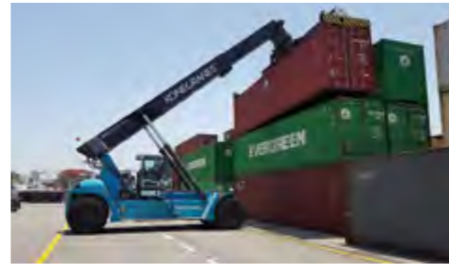
REACH STACKERS FOR CONTAINER HANDLING 10 – 45 TONS We offer the widest and deepest range of reach stackers for empty and laden container handling in container ports. You will find the capacity/performance ratio and feature list you need in our range.
