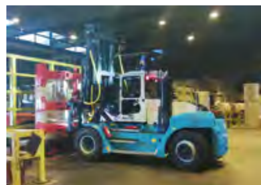
FORK LIFT TRUCK WITH DOUBLE PAPER CLAMP mounted on fork shaft. Lifts up to 6 reels across 2 rows in one lift. Seen here with a duplex free-lift mast, built low. Capacities 10–20 tons, optional rotator, bale clamp and tilt.
