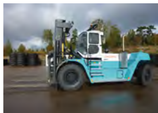
FORK LIFT TRUCK WITH MULTIPLE MAST COMBINATIONS. Duplex mast with or without free-lift. Triplex mast, several fork carriages and fork types available. Capacities 10-65 tons.
