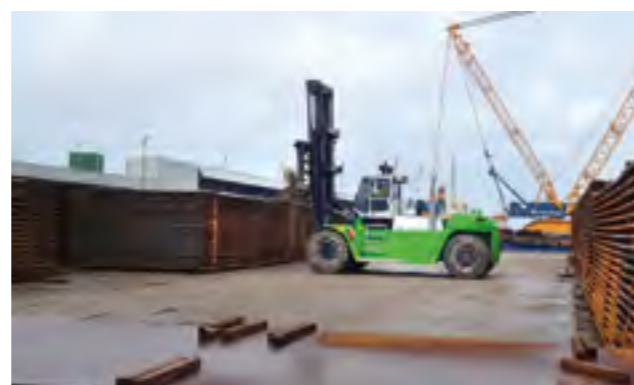
FORK LIFT TRUCK CUSTOMIZED FOR WIND POWER HANDLING of large, thick steel plates for tower section manufacturing. Very strong lifting equipment and reinforcement. Capacities 25–65 tons.
