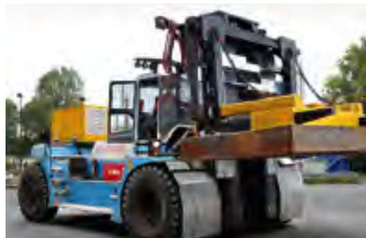
HEAVY-DUTY FORK LIFT TRUCK with magnet. Powered by diesel generator. Special equipment for handling steel slabs.
