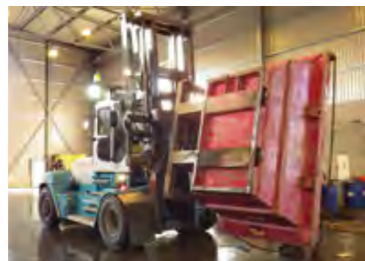
FORK LIFT TRUCK WITH 360 DEGREE INTEGRAL ROTATOR for waste-to-energy and biomass handling. Capacities 10–25 tons.
