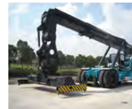
SPECIAL REACH STACKER . Alpro, food and drink products, Wevelgem, Belgium. This customer had very special requirements, needing a barge handler but having very serious limitations on ground pressure. Alpro is very strongly focused on safety and green technology. This was one of the first lift trucks with AdBlue technology delivered to Belgium. Due to the limitations on ground pressure, we delivered an SMV 4542 TBX4 BH reach stacker with a 7500 mm wheelbase and a larger than standard jack plate to reduce ground pressure. It's equipped with a heavy-duty boom for barge handling. It has many safety extras: reverse distance control, laser-based distance measuring system, lots of extra lamps, and so on. The customer is very satisfied with the truck and the advice and support given during the purchasing procedure. We were the only manufacturer that could supply this kind of custom-built machine.
