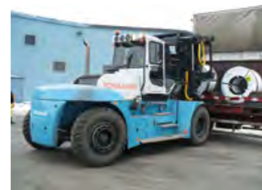
FORK LIFT TRUCK WITH FREE-LIFT MAST, fork-shaft system and single coil ram, handling automotive steel and aluminum coils.
