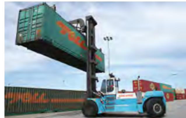
LADEN CONTAINER HANDLERS 33 – 45 TONS Konecranes laden container lift trucks offer a fast total operating speed (lifting + lowering + driving speed). The ratio of lifting capacity to truck size and length is best-in-class. These heavy-duty top-loaders are very stable and still compact.
