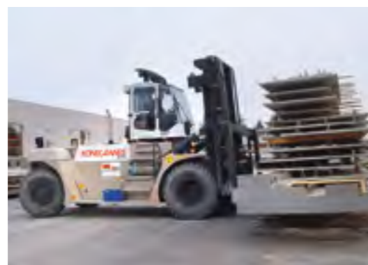
HANDLING OF CONCRETE SECTIONS , fork lift truck with wider carriage, long forks, elevated cabin and reinforced lifting equipment, SMV 25-1200 C and 33-1200 C.
