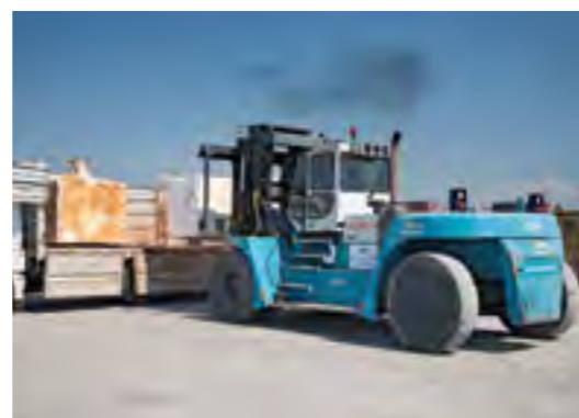
Big marble blocks, 5–30 tons , loading and unloading trucks and containers, SMV 25-1200 C and 33-1200 C.
