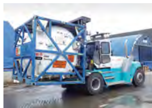
HANDLING 5-, 10- AND 20-FT SPECIAL TANK CONTAINERS with fork pockets, on oil and gas frames, fork lift truck models SMV 10-600 C and 16-1200 C.
