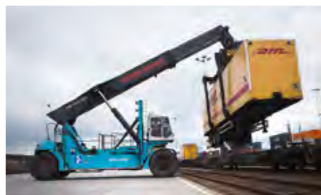
INTERMODAL HANDLING IN THE PORT OF HELSINGBORG , with 4 rail tracks 650 m long and 2 rail tracks handled from both sides. This big stacker lifts 45 tons across all three container rows and both rail tracks. It has an elevating cabin and can be controlled remotely.
