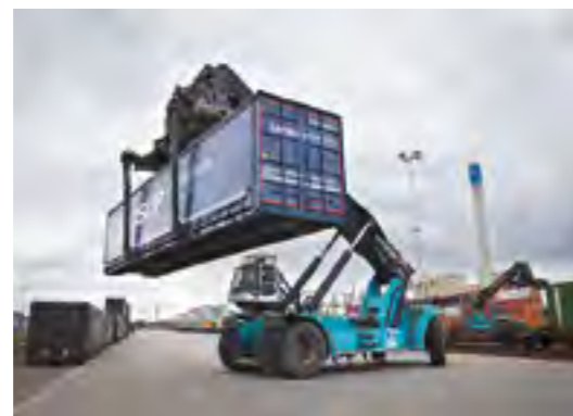
REACH STACKER AND SPREADER WITH OVERHEIGHT FOLDING LEGS for handling containers with open tops for overheight cargo.
