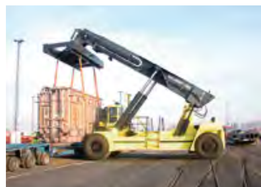
EXTRA-LARGE REACH STACKER WITH SLINGS to lift various kinds of special things e.g. machinery, wind turbine components weighing up to 80 tons with a load center of 2500 mm.
