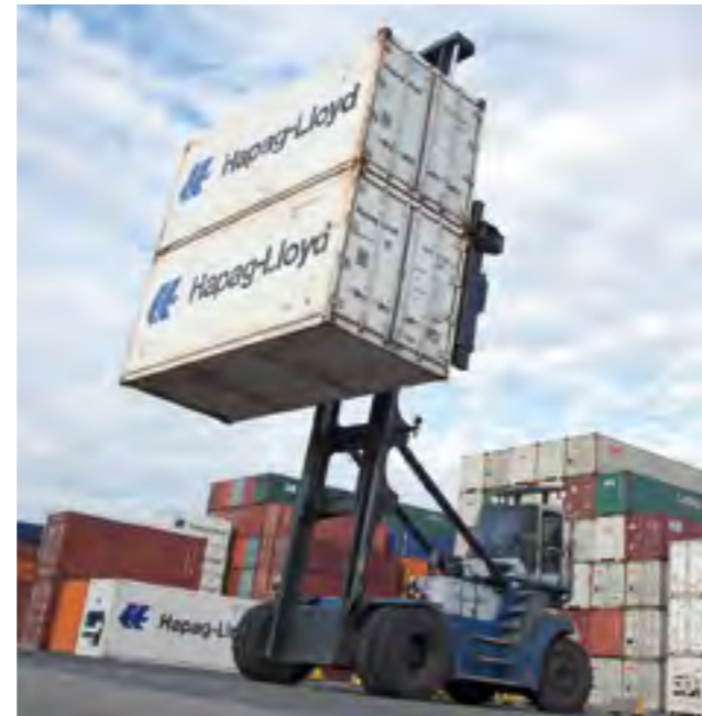
EMPTY CONTAINER HANDLERS 8 – 10 TONS Konecranes empty container lift trucks offer a very fast total operating speed as a function of lifting, lowering and driving speed. Our range has mid-mounted and rear-mounted cabins and excellent stability.
