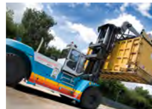
LADEN CONTAINER LIFT TRUCK for waste-to-energy and biomass container handling. Capacities 25–45 tons.
