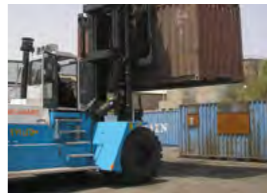
FORK LIFT TRUCK HANDLING CONTAINERS LOADED WITH AUTOMOTIVE COMPONENTS including engines, transmissions, etc. Capacities 16–42 tons.
