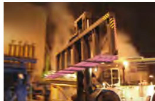
FORK LIFT TRUCK, CAPACITY 60 TONS, handling hot steel slabs, blooms and billets with temperatures up to 800 degrees. Special attachment, carriage 11 m wide with 7 forks, to ensure that the steel does not bend during hot transport. Reinforced lifting equipment and heat protection. Capacities up to 60 tons.
