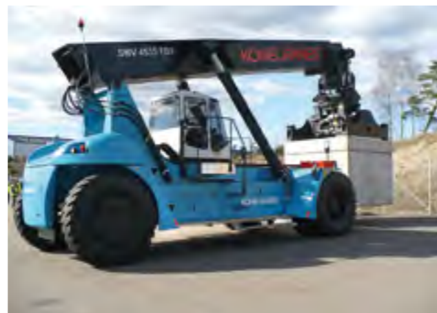
KONECRANES HAS SUPPLIED A SPECIAL REACH STACKER to handle 45-ton concrete overpacks containing intermediate level nuclear waste (ILW) for Magnox North at its Trawsfynydd site in Wales.
