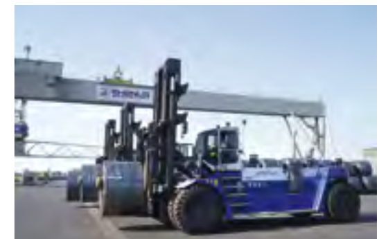
FORK LIFT TRUCK WITH FORKS MOUNTED ON A FORK SHAFT. Quick-change fork shaft makes it possible to swap quickly between e.g. coil rams and lifting magnets.
