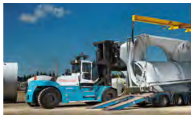
FORK LIFT TRUCK CUSTOMIZED FOR WIND POWER HANDLING, from steel plates to tower sections to generator housings and windmill blades. Capacities 10–65 tons.
