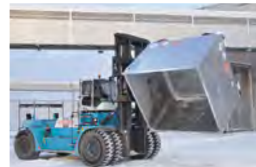
FORK LIFT TRUCK WITH INTEGRAL 360-DEGREE ROTATOR for scrap handling in containers with fork pockets. Capacities 10–60 tons.
