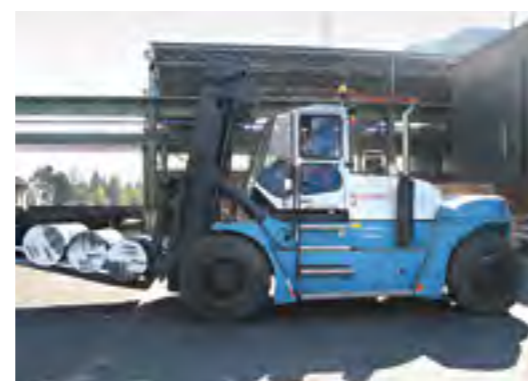
FORK LIFT TRUCK FOR STEEL OR ALUMINUM MILLS handling ingots, slabs and melting pots with special reinforcement and heat protection for hot metal handling. Capacities 10-65 tons.
