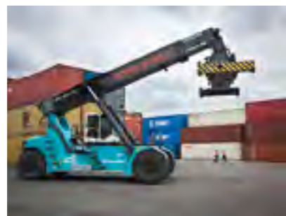
TC hydraulic sliding cabin Stroke 2900/3300 mm
