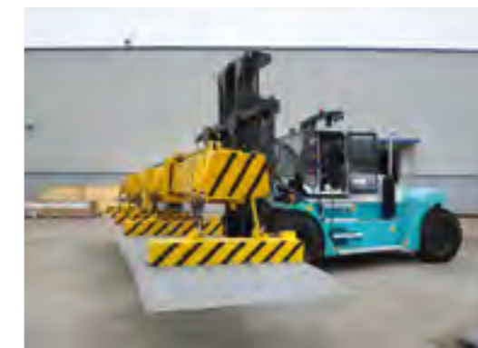
FORK LIFT TRUCK WITH FORK-MOUNTED MAGNET, handling 1–20 mm steel plates.
