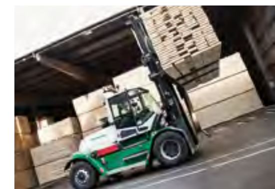
12-TON FORK LIFT TRUCK moving sawn wood bundles at a sawmill.
