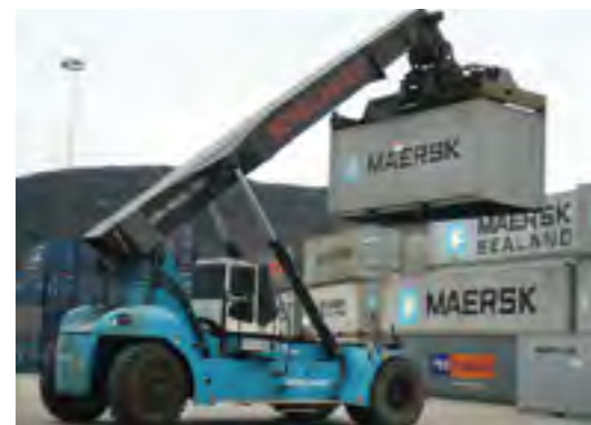
REACH STACKER FOR AUTOMOTIVE LOGISTIC OPERATIONS. Various models for handling 20–45 ft containers, auto body parts, engines, transmissions and other automotive components.
