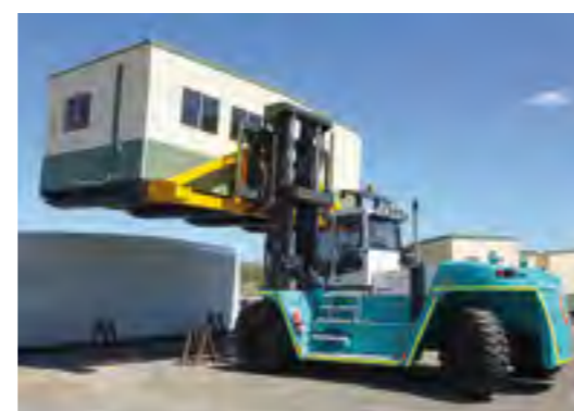
HANDLING PRE-FABRICATED office unit. Various mast and fork combinations possible.
