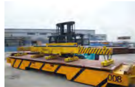
FORK LIFT TRUCK WITH MAGNET ATTACHMENT for handling steel plates and slabs. Can be expanded to various widths 3–13 m.
