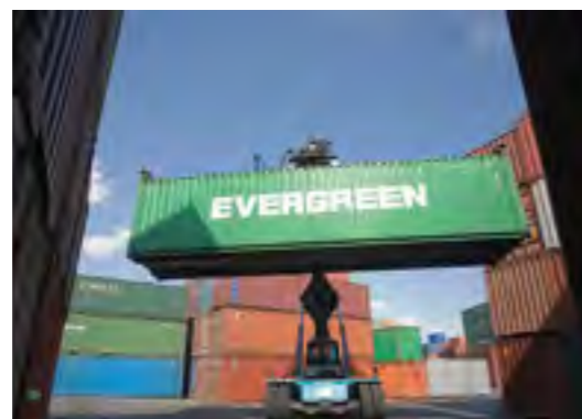
REACH STACKER FOR EMPTY & SEMI-LADEN CONTAINER HANDLING , stacking up to 3 or 6 containers high and 10 or 25 tons in the first row. Very efficient operation: the reach stacker can rotate the containers 300 degrees.
