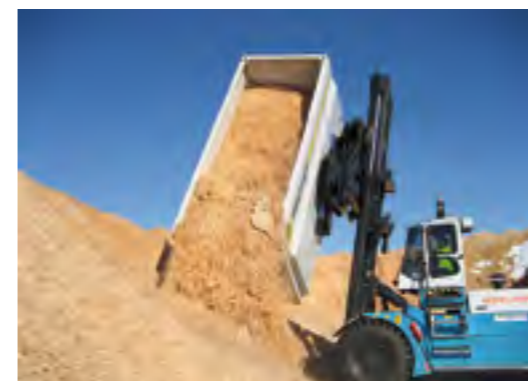
FORK LIFT TRUCK WITH 360 DEGREE INTEGRAL ROTATOR for biomass and waste-to-energy handling. Capacities 33–45 tons.
