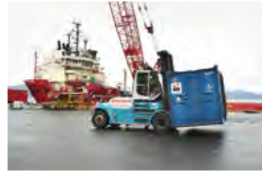
HANDLING 5-, 10- AND 20-FT SPECIAL TANK CONTAINERS with fork pockets, on oil & gas frames, fork lift truck models SMV 10-600 C and 16-1200 C.
