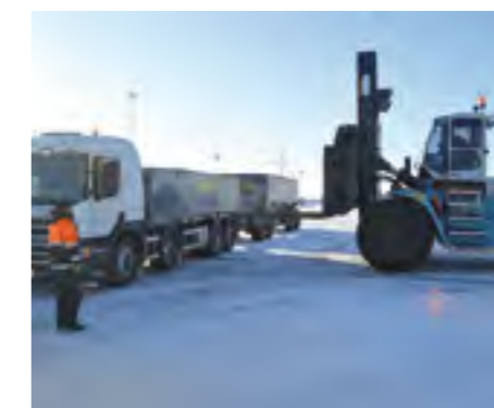
SMV 45-1200 FORK LIFT TRUCK working in a mining application, Valtasiirto Oy, Finland. A multi-functional truck with forks, fork rotator (360 degrees) and a container spreader.
