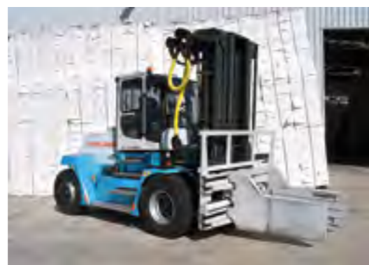
FORK LIFT TRUCK WITH EXPANDABLE PAPER BALE ATTACHMENT mounted on fork shaft for e.g. paper recycling operations. Lifts multiple bales in one lift. Capacities 10–20 tons, optional rotator, bale clamp, tilt.
