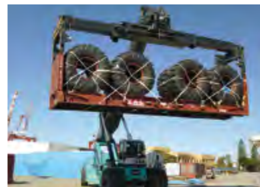
REACH STACKER WITH FOLDABLE LEGS handling big tires on flat racks.
