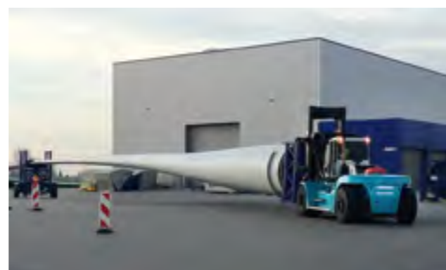
FORK LIFT TRUCK BUILT TO HANDLE LONG WIND BLADES from 20–65 m. Capacities 10–33 tons.
