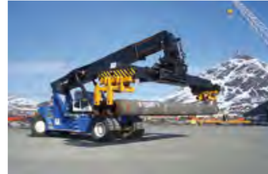
HANDLING BIG PIPES, VARIOUS SIZES AND WEIGHTS with a regular reach stacker equipped with a pipe clamp attachment. One to five pipes can be lifted at a time, weighing 1–30 tons.
