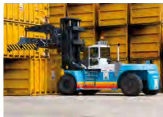
WASTE IS HANDLED MAINLY IN 20-FT CONTAINERS that are transported by road, rail or water. They can be handled by fork lift trucks, laden container lift trucks (seen here) or reach stackers. Waste containers weigh from 15–25 tons.
