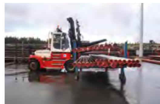
PIPE-HANDLING FORK LIFT TRUCK WITH A HYDRAULIC PIPE CLAMP can safely handle long pipes. Capacities 10–45 tons.
