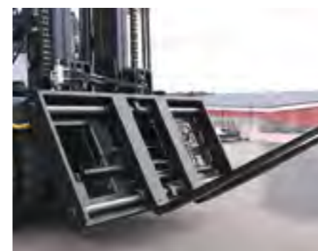
SMV 10-1200 FORK LIFT TRUCK owned by Heléns, a tubing/piping warehousing company in Halmstad, Sweden. Specially equipped for handling long steel pipes: extra big tilt for long goods of ±30 degrees.
