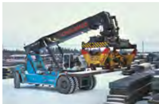
REACH STACKER FOR COMBINED CONTAINER AND STEEL SLAB HANDLING. The hydraulic grab attachment lifts 1–3 slabs of up to 40 tons in one lift. A multi-function stacker.
