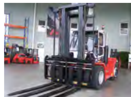
SMV 12-600 B FORK LIFT TRUCK owned by dealer Suffel Fördertechnik GmbH, Germany. Double pallet handling with four forks for dairy and brewery products.
