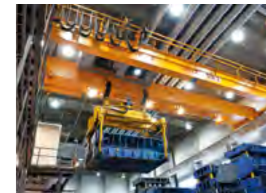
INDUSTRIAL CRANE lifting stamping press tools.
