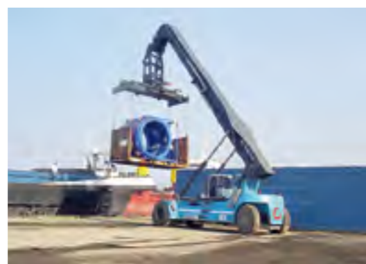
REACH STACKER LIFTING OVERHEIGHT FLAT RACKS with slings. Seen here: loading turbines and generators onto river barges. Capacities up to 45 tons.
