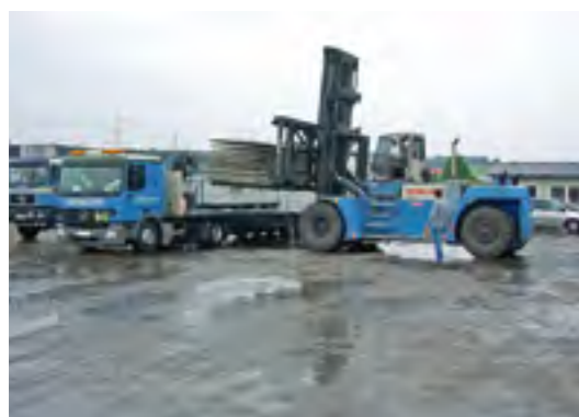
BRICK PRODUCTION , handling of single and double brick packages with integral hydraulic gripper. Capacities 10–20 tons.
