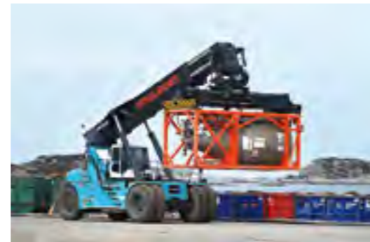
REACH STACKER LIFTING SPECIAL TANKS and offshore equipment.
