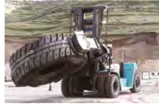
FORK LIFT TRUCK WITH TIRE HANDLING ATTACHMENT , handling tires from 2-5 m in diameter and loads weighing up to 20 tons. Truck models SMV 16-1200 C to 42-1200 C.
