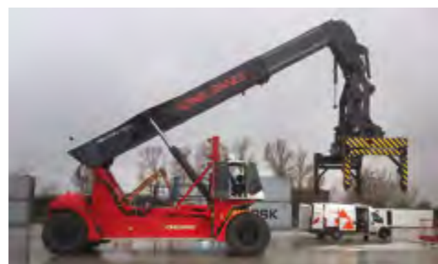
THIS REACH STACKER DOES BARGE CONTAINER HANDLING at the Terminal de Seine in Paris. It has a movable cabin that gives the driver good sightlines and a spreader with overheight folding legs.
