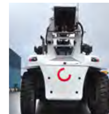
SMV 4537 TBX6 "NEW COMBINATION" REACH STACKER . Faroe Islands, owned by Eimskip, the Icelandic Steamship Company. This reach stacker can handle tank containers up to 14 tons into the 4th container row at load center 8.75 m. It lifts 6 high in the 1st row, capacities 45-40-27-14 tons (with jacks) for rows 1-to-4. We mounted a boom designed for a larger reach stacker on this small truck body in order to meet the customer's requirements.
