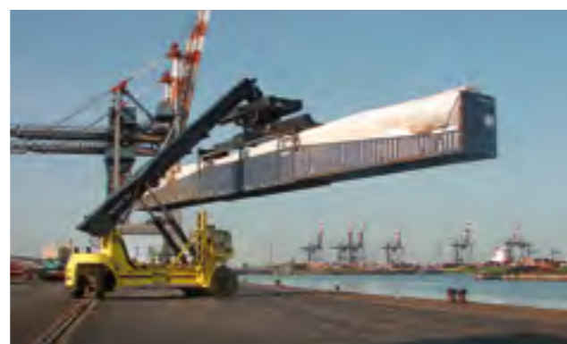
KONECRANES REACH STACKERS, LIFTING CAPACITIES 45/80 TONS, seen here handling long wind turbine blades in Germany.
