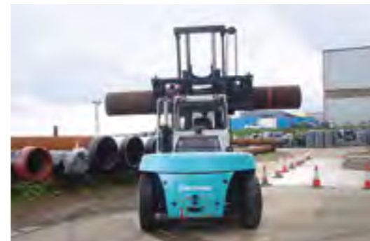
ONE BIG PIPE OR MULTIPLE SMALLER PIPES can be handled with a hydraulic pipe clamp attachment. Capacities 10–45 tons.
