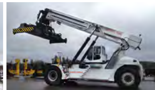
SMV 4537 TBX6 "NEW COMBINATION" REACH STACKER . Faroe Islands, owned by Eimskip, the Icelandic Steamship Company. This reach stacker can handle tank containers up to 14 tons into the 4th container row at load center 8.75 m. It lifts 6 high in the 1st row, capacities 45-40-27-14 tons (with jacks) for rows 1-to-4. We mounted a boom designed for a larger reach stacker on this small truck body in order to meet the customer's requirements.
