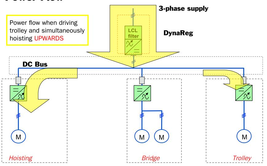
**Network Braking System Power Flow**
